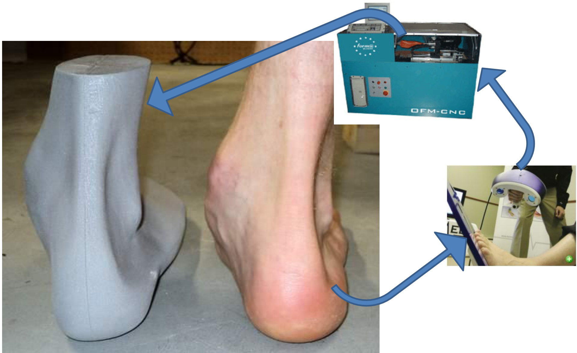
Picture Comparison of the actual foot to the same foot 3D video laser scanned and CNC milled out of PU foam (grey)
